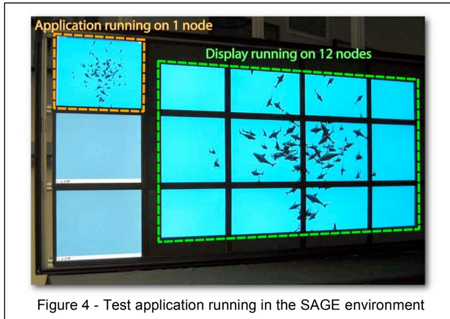
Figure 4 - Test application running in the SAGE environment
